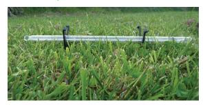
• Its construction and working is similar to that of minimum thermometer except that its bulb is spherical and the stem is encased in a glass jacket in order to protect seal marks on the stem from dew, rain.
