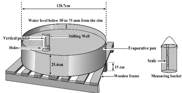
Fig: Components of Class A pan Evaporimeter
